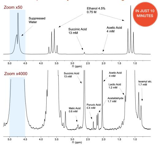
The Spinsolve 80 ULTRA is ideal to study biochemical processes like fermentations. The high sensitivity of the 80 MHz model makes it possible to detect metabolites produced at sub millimolar concentrations in just minutes. In this particular example, solvent suppression was combined with carbon decoupling to eliminate the carbon satellites of the NMR signals of ethanol produced during the fermentation process.
